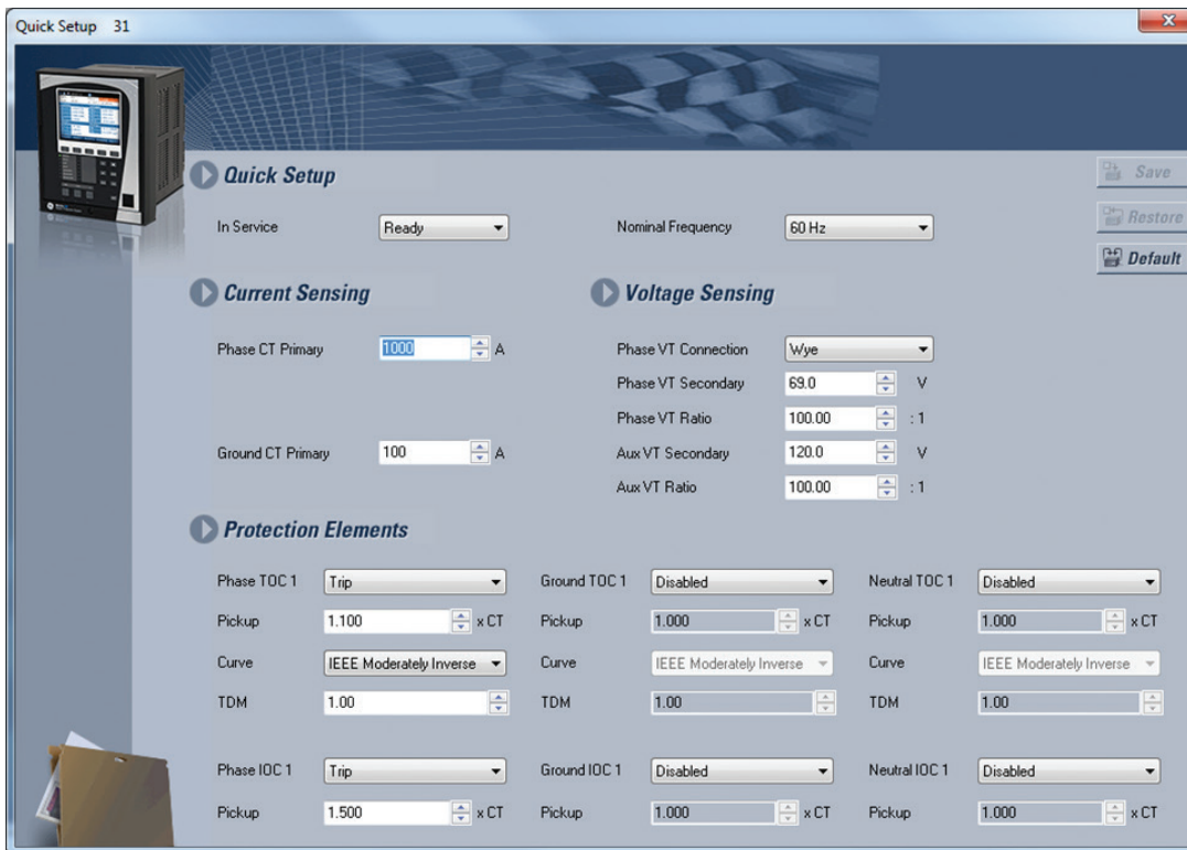
Figure 3. Quick setup options allows setup and configuration of the Multilin 850 in few easy steps.
