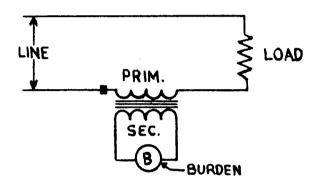
Current transformers having tapped secondaries are referred to as double-rated, tapped secondary CT's. They are used in applications where it is necessary to have available two ratios of primary to secondary current from the same secondary winding of the CT. This may be accomplished by adding a tap in the secondary winding to get a second ratio. The ratio obtained by the tap is usually one-half the ratio obtained by the full secondary winding. A schematic example is shown below.
