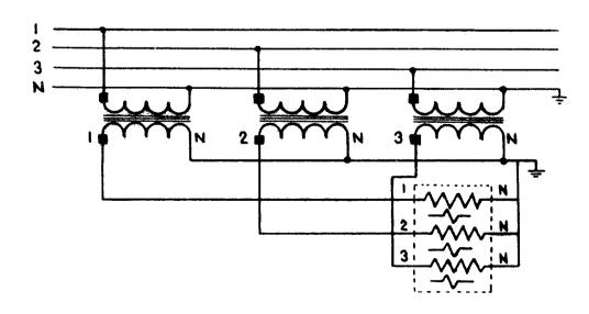
Note the polarity markings and their relationship to one another as well as the watthour meter potential coils. It also should be noted that the secondary windings are grounded at a common junction.
