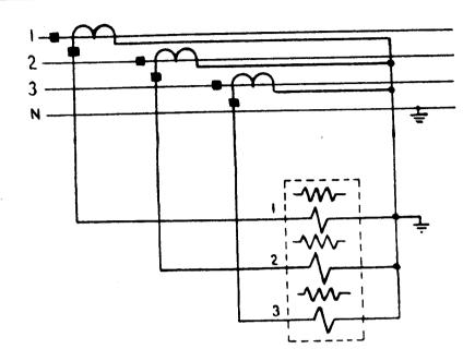
Note particularly the relationship of the polarity markings to one another and to the instrument terminals. As was previously shown for potential transformers, the current transformers should also have their secondary windings grounded.
