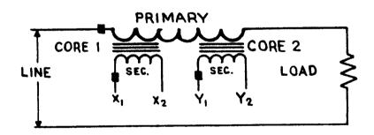
In this design, if both the circuits are not going to be used simultaneously, then the unused circuit <u>must be</u> short circuited while the other is energized or again you will develop an induced high voltage on the open circuited unused portion as pointed out previously.
