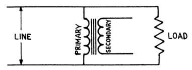
When a phase relationship of "direction of flow" is of no consequence, such as in a voltmeter which operates only according to the magnitude of the voltage, there is no need to observe the polarity of the transformer. However, in watthour meter applications, polarity must always be observed.
