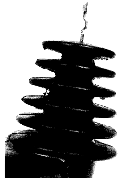
Westinghouse VOZ-20 Bushing with Molding "Flash" Evident on Skirts.
