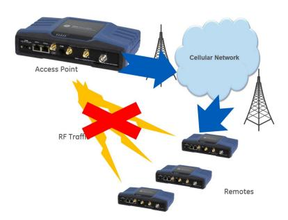
If a failure event occurs that prevents communication over the RF Network traffic would automatically be sent over the cellular network.
