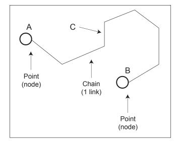
In the Smallworld view of the world the two switches A and B are represented by what are called points. Each point is linked to a single node that stores its geographic location. The cable C is represented by what is called a chain. In this example, it consists of a single link. This link holds the route of the cable and also represents its connectivity.
