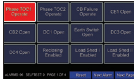
12 to 48 user-configurable alarms per page eliminate the need for a separate annunciator.
