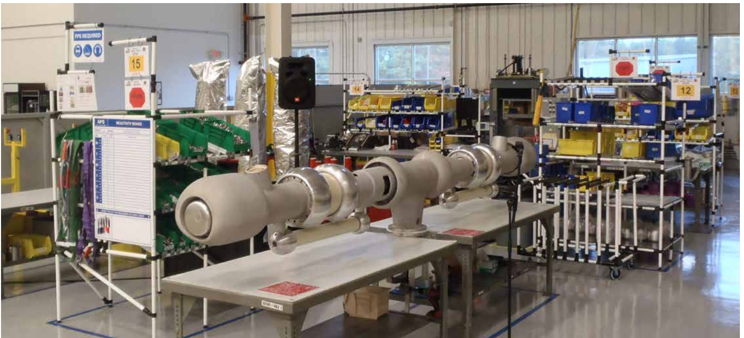
Assembly of interrupter - 550 kV interrupter in a clean room environment.
