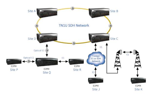
Remote E1MX Multiplexers (Add/Drop) are connected to a TN1U SDH network over an E1 link. DSO channels from Sites P and R are consolidated at Site Q and groomed for E1 connection to Site D.
