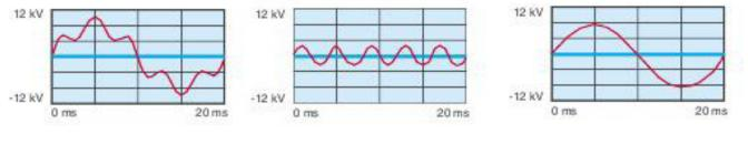
1. Voltage waveform distorted by 5th harmonic.
