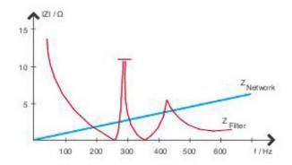
This problem could not have been solved by the use of capacitor banks without reactors or with damping reactors, because the resulting parallel resonance would have amplified the harmonics and exacerbated the distortion problem.
