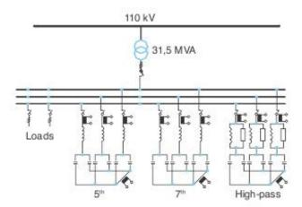
Figure 2: 5th, 7th and high-pass filter
