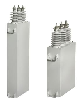
The dielectric liquid is specially made for capacitor units and has been chosen by Grid Solutions for its excellent electrical properties and heat stability at both low and high temperatures. It is non-PCB, non-chlorine and biodegradable.
