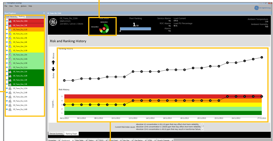
The risk index ring shows the varying risk index stages the transformer has been in over a 9 month period, with the current risk index in the center.
