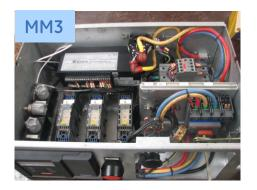
Once the MM3 unit is removed, a supporting plate is installed in the chassis using the existing MM3 mounting holes. A DIN rail is then installed to support the MM300
