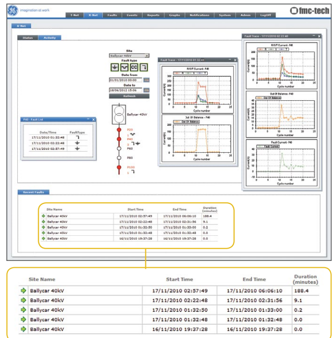
Support maintenance prioritization based on fault history activity for feeder segments
