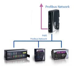
Connect multiple Modbus devices to a Profibus Network
