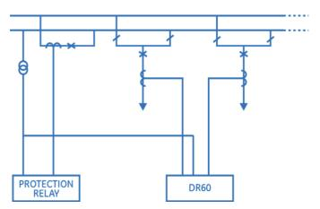
The DR60 can be installed to monitor and record analog and binary signals. Depending on the part number option, with a single DR60 it is possible to have: up to 32 analog inputs; up to 96 binary inputs; up to 32 high-speed transducer inputs for HVDC or up to 48 binary outputs.
