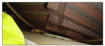
**Findings:** Short circuit and circulating current damages identified on core and core frame of a 19 year old large step down transformer 230 kV/10,5 kV.
