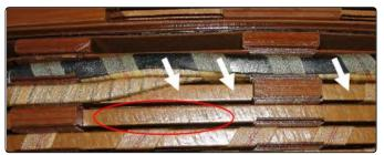
**Figure 3:** Paper sampling locations must be chosen according to the accessibility and rebuilt feasibility. Locations should be reasonably representative of winding temperature conditions or hot spot conditions.
