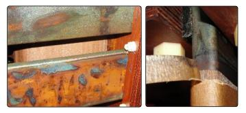
**Findings:** Copper sulphide formed on copper busbar and in the wraps of the paper insulation on copper conductors.
