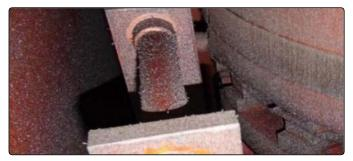
**Findings:** Sludge formation and aggregated particles aligned in a direction perpendicular to the surface, following the localized electrical field gradient.
