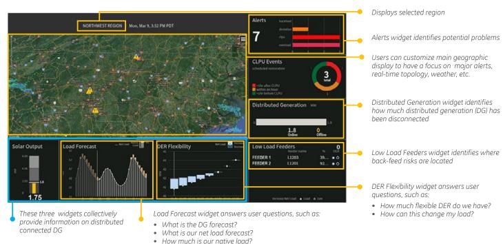
Grid IQ Insight enables a utility with low visibility into their network to use irradiance data and their distribution connectivity model to understand real-time DG contribution versus its native load. Grid IQ Insight delivered an understanding of both the utility's DG flexibility and their resource adequacy for restoration following system disturbances.
