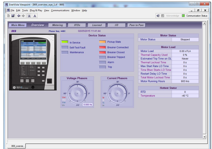
View motor status using digital inputs, analog inputs and RTD inputs.
