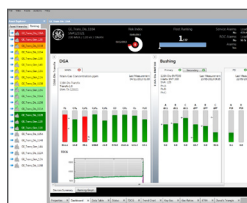
Transformer health/risk overview
