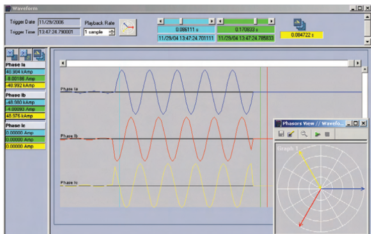
Use the oscillography feature as an accurate troubleshooting and diagnostics tool
