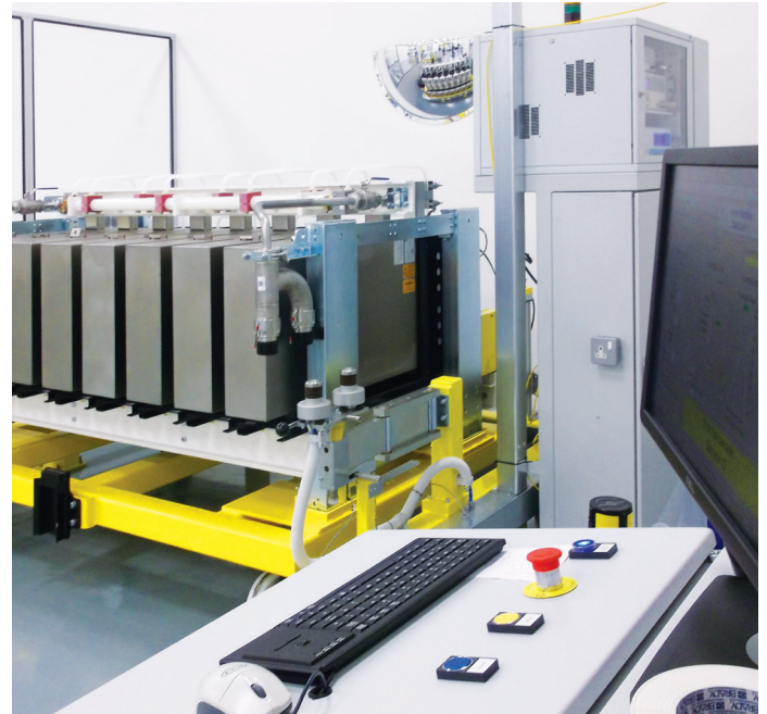
VSC module end of line production test
