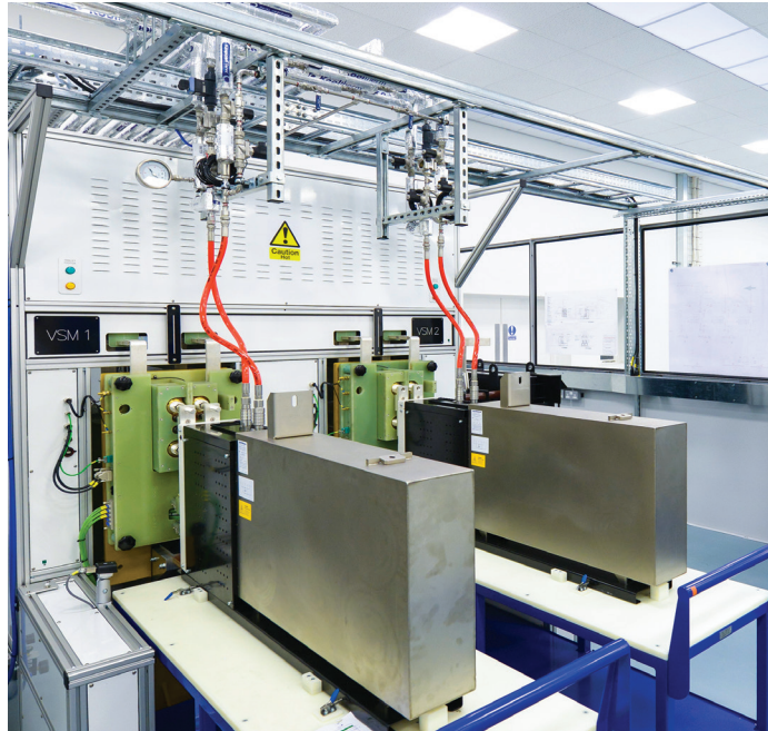
VSC sub module end of line production test
