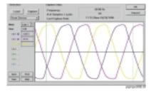
Event Recorder: alarms, setpoint triggers, input and output events can be stored in a 40 event record and time and date stamped by the internal clock. This is useful for diagnosing problems and system activity. Minimum and maximum values are also continuously updated and time stamped.
