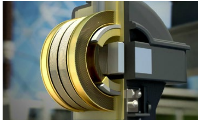
Lattice-type winding in a JVS350 station-class VT
