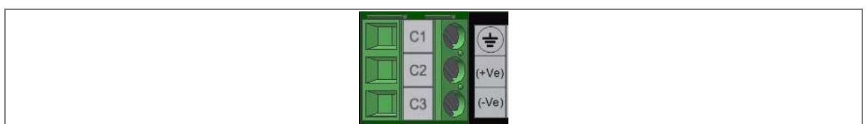
Figure 9: Earthing terminal on the rear side of the relay
