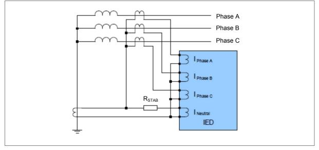
Figure 12: High Impedance REF connection
