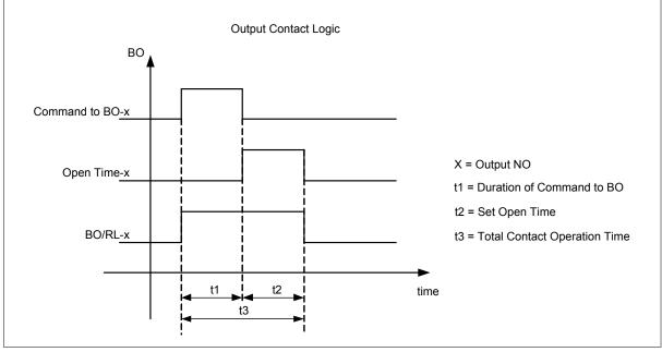
Figure 2: Output contact logic
