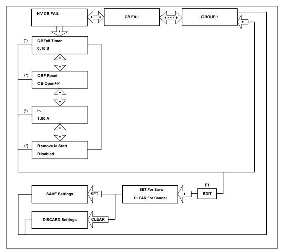
Note: (\*) indicates **EDIT** key used to modify settings. Refer to the View and Edit settings section. LV CB Fail settings can be done in similar manner as HV CB Fail settings
