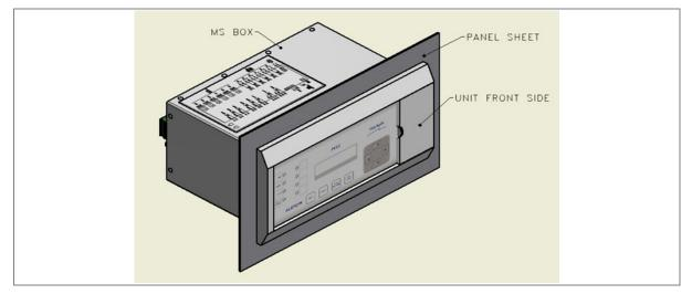
Figure 1: Inserting relay in to the panel cutout
