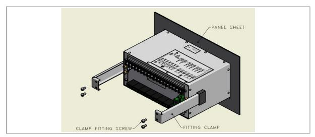
Figure 2: Tightening fitting clamps
