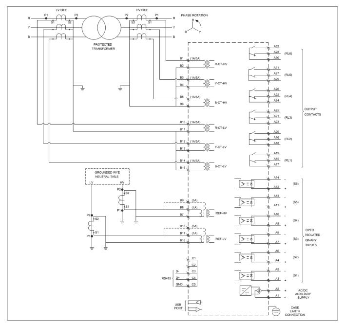
Figure 1: P652 wiring diagram
