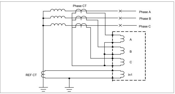
Figure 10: CT connection diagram for low impedance REF application
