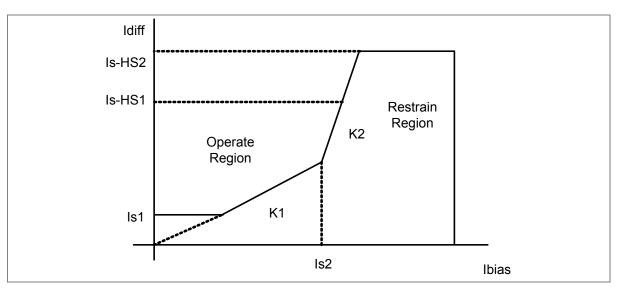
Figure 6: Transformer Differential operating characteristics
