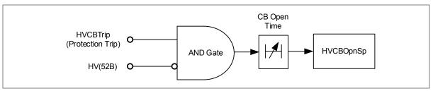
Figure 6: HV CB open supervision logic
