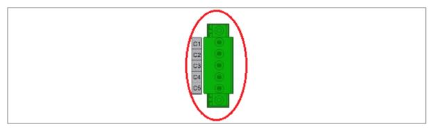
Figure 7: Rear serial port terminal block
