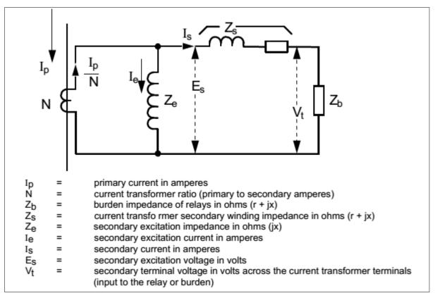
Figure 2: CT equivalent circuit
