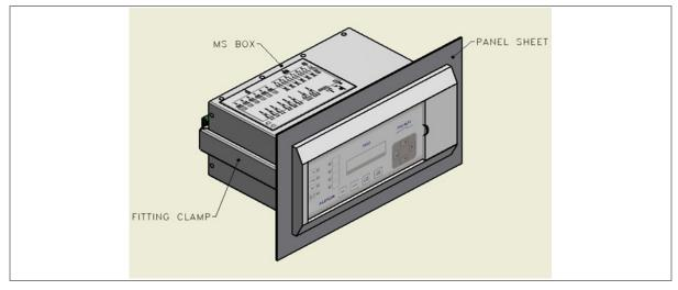
Figure 3: Relay mounted on the panel-front view
