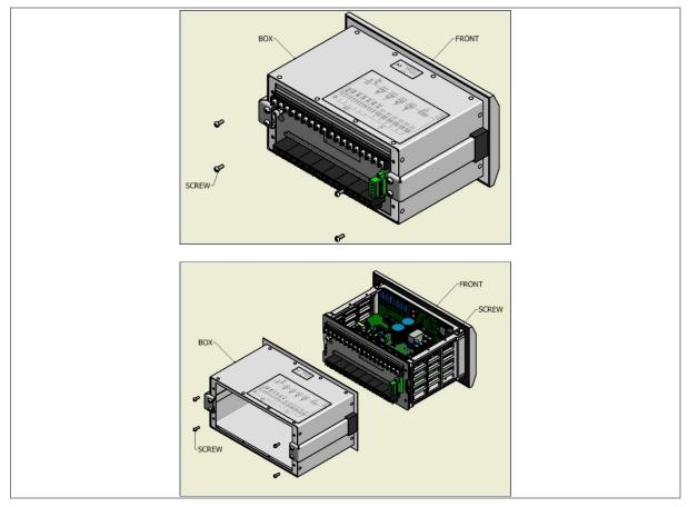
Figure 1: Removal of relay cover
