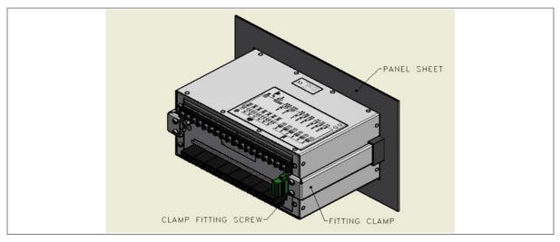
Figure 4: Relay mounted on the panel-rear view
