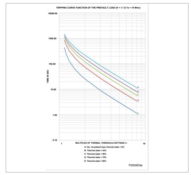
Figure 13: Thermal Overload curve
