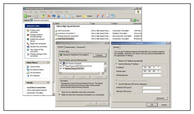
With the PC set to Local Area Connection and the device connected it is necessary to set an IP address in the device. Using the 'Browse Ethernet Devices' function (section 9.4) the product will not be found unless it has been previously assigned an IP address in the required range.
