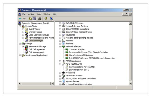
A RS232 port will show as 'Communications Port' and the USB to RS232 converter will be identified along with its installation COM port.
