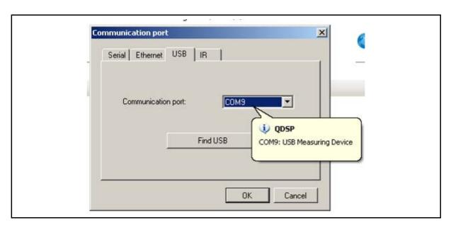
When 'Find USB' is selected the software will report which USB COM port is connected to an iSTAT product, as shown above. The balloon message will only remain for a few seconds. The USB COM port reported as connected to the iSTAT product will be loaded as 'Communication port', press 'OK' to continue.
