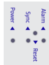
Figure 17: Local HMI from RT431
