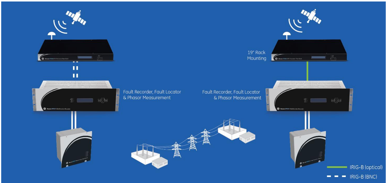
Figure 38: TWFL application using RT430/434 for Time Sync
