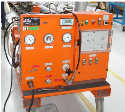
Figure 8 – Vacuum filling gas plant DILO and connecting valves
