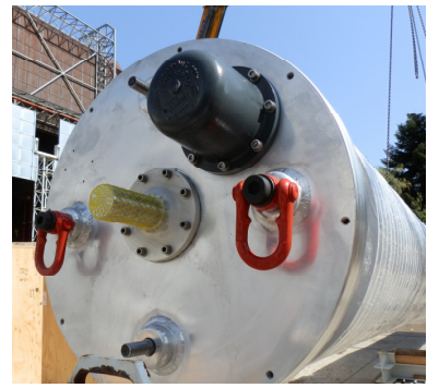
Figure 6 – Example of lifting hooks on main flange and on outdoor and indoor sides extremities
