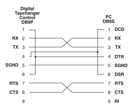
Figure 9-36 Null Modem Cable 9-Pin to 9-Pin
