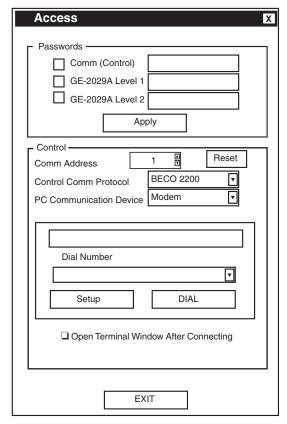
Figure 9-11 Communication Access (Modem) Dialog
