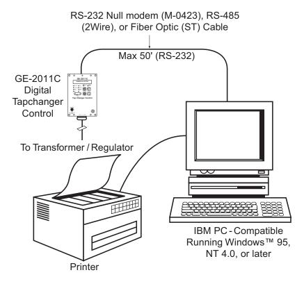
Figure 1 Direct Connection
