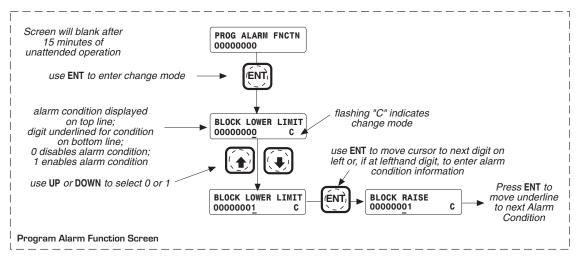
Figure A-6 Programmable Alarm Function Screen
