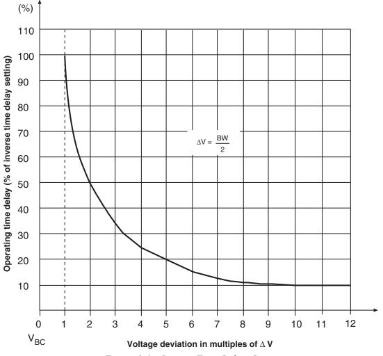
Figure 3-1 Inverse Time Delay Curve
