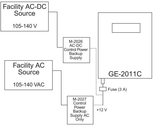
Figure 6-5 Typical Control Power Backup Connection for GE-2011C
