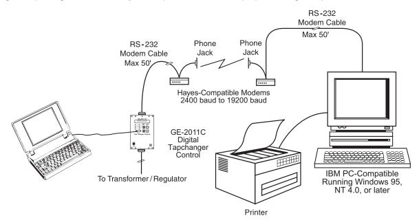
Figure 2 Modem Connection
