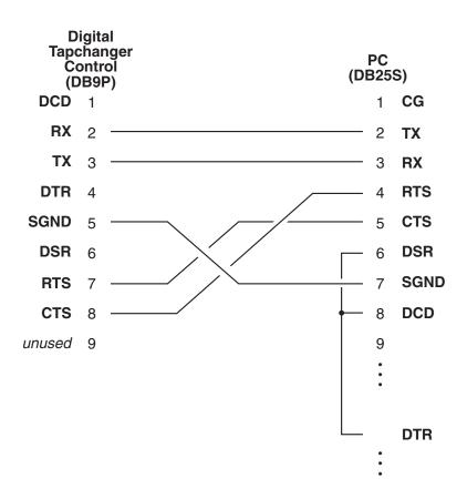
Figure 9-37 Null Modem Cable 9-Pin to 25-Pin
