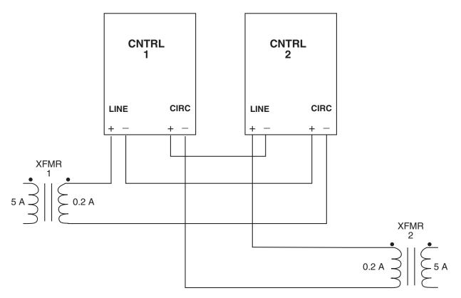
Figure 4-4  $\triangle VAR2$  Paralleling
