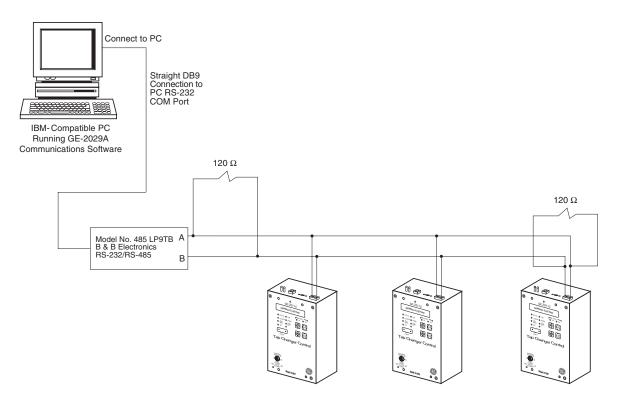
Figure 5 RS-485 Network Connection
