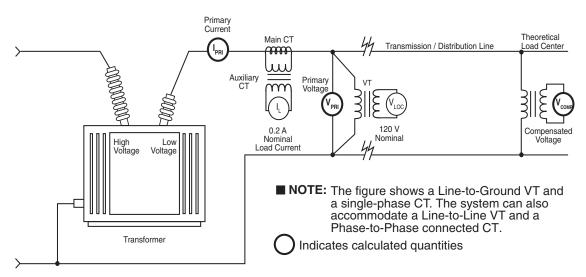
Figure 5-2 Secondary Quantity Metering and Primary Quantity Calculations for Transformer Applications
