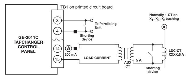
Figure 8-18 GE-2011C Group B-1005 Wiring Harness Setup for Current Checkout Procedure
