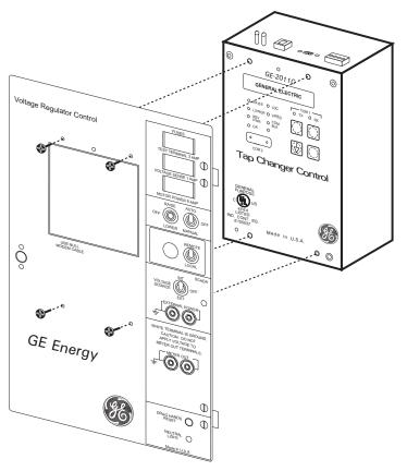
Figure 1-2 Typical Adapter Panel Mounting
