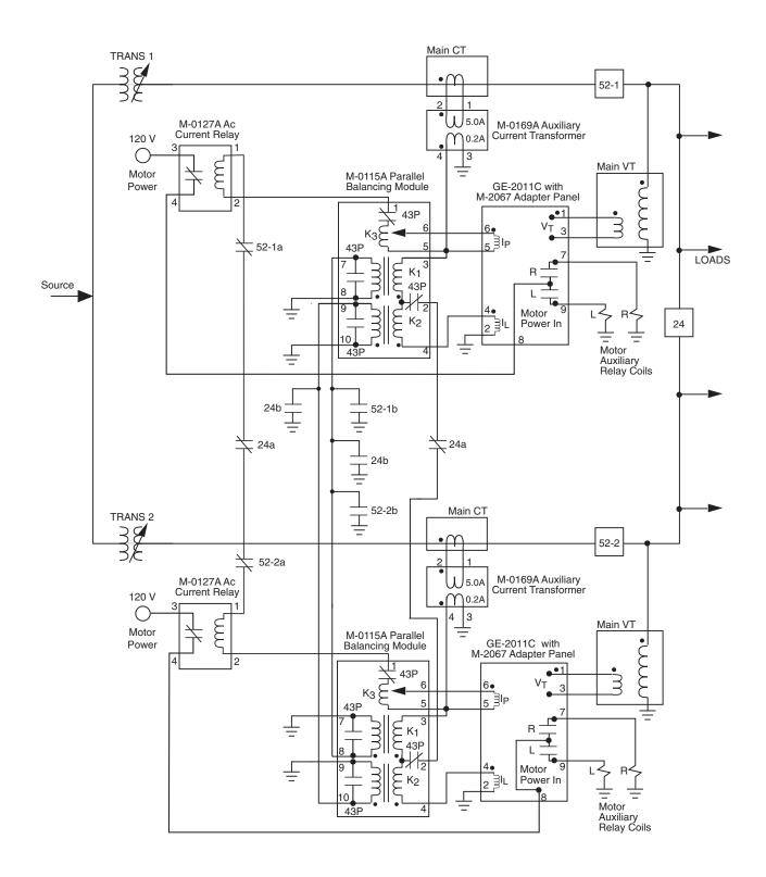
Figure 4-2 GE-2011C and M-2067 Paralleling Scheme for Two Transformers using the Circulating Current or  $\Delta VAR^{TM}$
