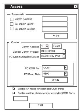
Figure 9-10 Communication Access (Serial) Dialog
