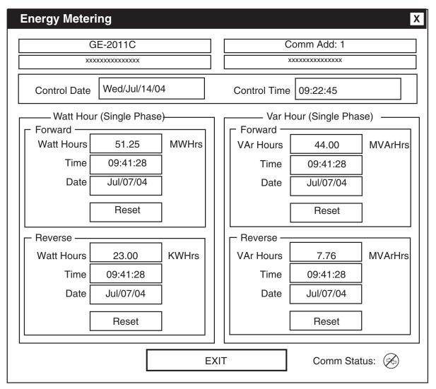
Figure 9-24 Energy Metering Screen
