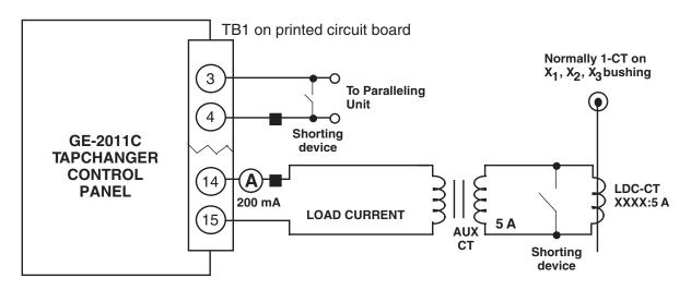
Figure 8-7 GE-2011C Setup for Current Checkout Procedure
