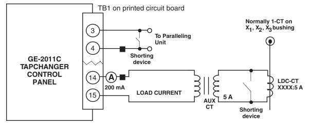
Figure 8-14 GE-2011C Setup for Current Checkout Procedure
