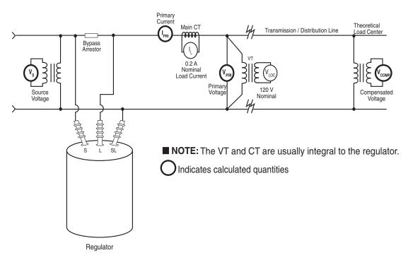
Figure 5-1 Secondary Quantity Metering and Primary Quantity Calculations for Regulator Applications
