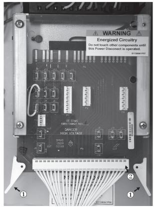
Figure 8-3 Power Disconnect Circuit Board
