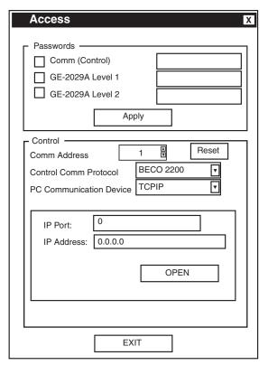
Figure 9-15 TCP/IP Communication Setup
