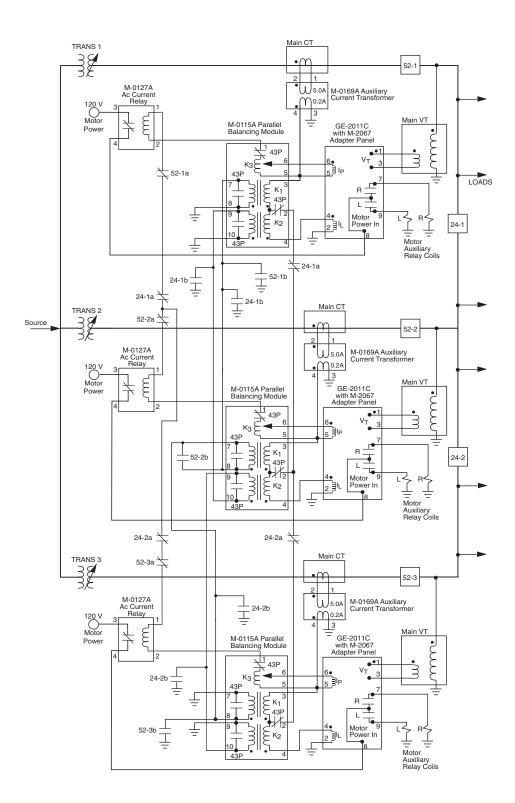
Figure 4-3 GE-2011C and M-2067 Paralleling Scheme for Three Transformers using the Circulating Current or  $\Delta VAR^{TM}$  Method
