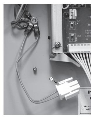
Figure 8-4 2-Pin Ground Connector
