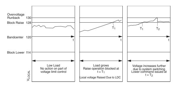
Figure 3-2 Local Voltage as Function of Load Current When Using Line Drop Compensation/ Action of Overvoltage and Overvoltage Runback Control
