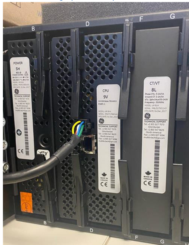
Figure 1: Black connector for graphical front panel above chrome connector
