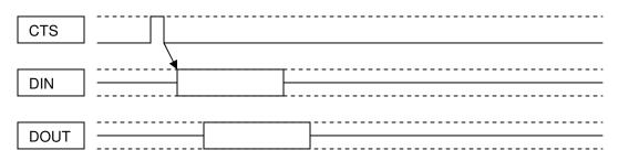
For half-duplex RCL vendor equipment, this can lead to problems in the case shown above because the radio is sending data out of the serial port at the same time data is coming in.
