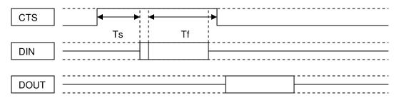
The MDS radio supports a half-duplex mode as follows. This mode is enabled with the command COM2 DUPLEX=HALF.
