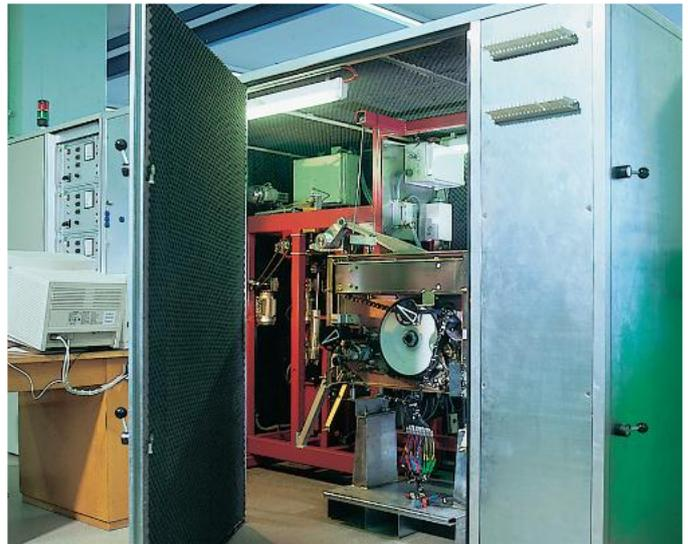
Spring mechanism routine test station
