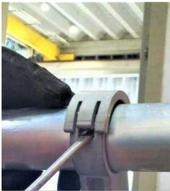
Figure 13: Removing lock cap with a screwdriver.
