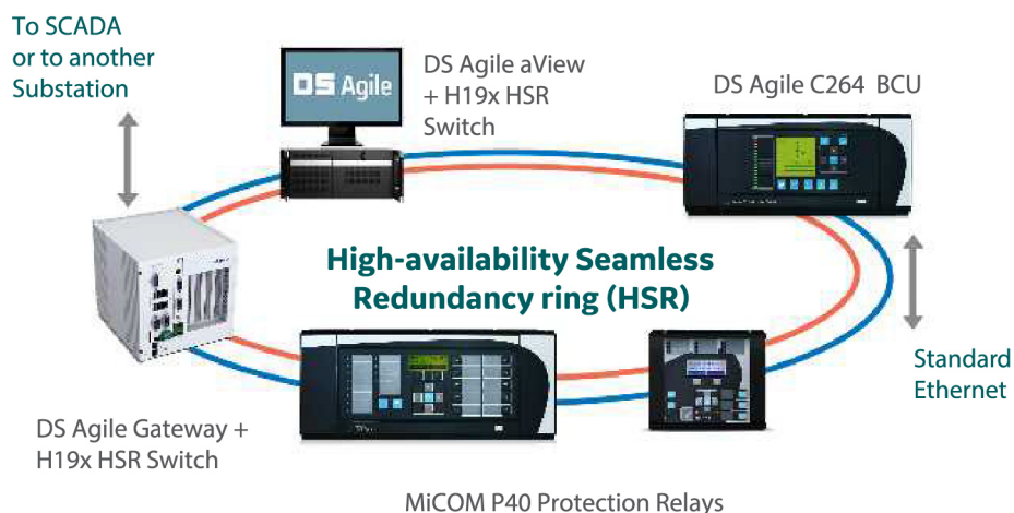
IEC 62439-3-5 HSR ring, Ethernet-based architecture
