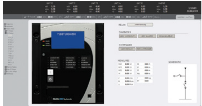
ECS HMI device screen detail
