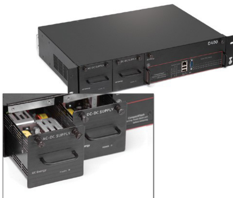
Redundant, hot-swappable power supplies.
