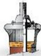
Fig. 7: Head of bushings 25 to 161 kV
