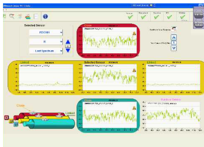
Neighbouring sensors monitored in the same view
