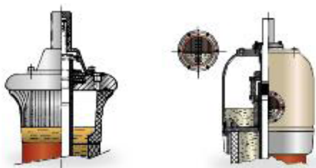
Fig. 3: Oil level indicator for prismatic glass and metal head
