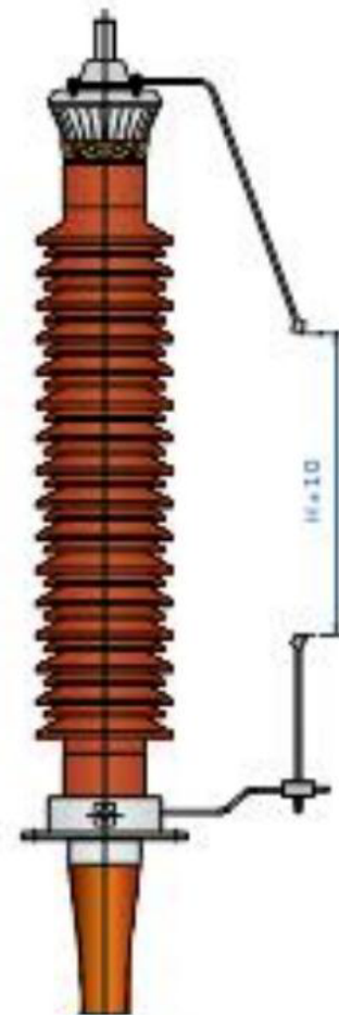
Fig. 6: Discharge distance for abushing equipped with arcing horns
