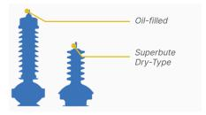
Even with their nice, compact size (up to 30% lower profile), Superbutes have more creep distance than oil-filled designs. This is an important factor in providing superior performance in coastal installations and other extreme environments.
