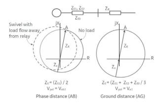
These characteristics are not fixed in size and vary proportionately with the source impedance directly behind the function. In the phase-distance (AB) diagram, load flow causes the characteristic to swivel to the left (as shown) or to the right relative to the forward reach (Point A). The amount and direction of the swivel depends on the magnitude and the direction of load flow.
