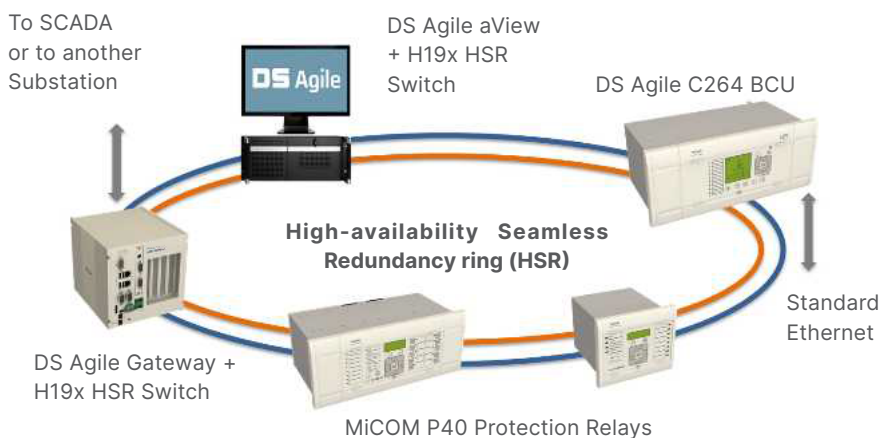
IEC 62439-3-5 HSR ring, Ethernet-based architecture
