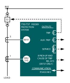
Ground level and time delay can be selected for coordination with upstream devices. The ground signal is normally derived as the residual sum of the three-phase CTs, eliminating the need for an additional ground sensor. Alternatively, for more sensitive detection, an additional core balance (zero sequence) ground sensor encircling the three-phase conductors can be used.
