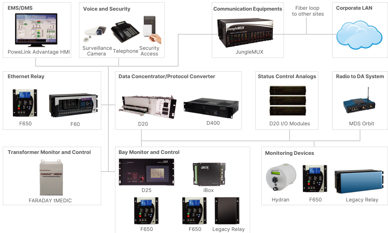
Figure 1: D20 Integrated Control System Connectivity
