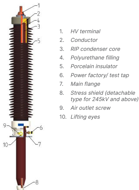
Fig. 4: PNR Bushing Typical Cross Section
