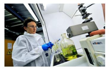
Oil samples are collected on site and analyzed by experts in our GE Vernova laboratories or by a local partner. Dissolved gas analysis on standard gases and complementary ones including oil quality, dielectric breakdown voltage, furans, moisture, and acidity can be performed. A report is generated that includes remedial actions and condition severity as per IEEE® or IEC® standards. Data can also be automatically transferred to the enterprise asset performance management system.
