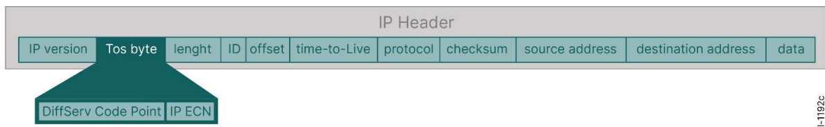
Figure 59: IP Header frame and Differentiated Service Code Point explained
