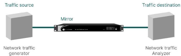
Figure 64: Port Mirroring in One Switch
