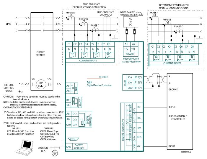
NOTE: For reference only. For connections for a specific MIF model, please refer to its external connections drawing.
