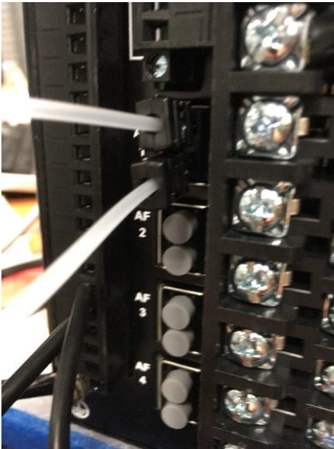
Figure 19. Loop Sensor Incorrect Installation;
