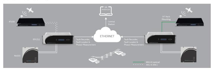
The solution is composed of the RPV311 processing unit, the RA333 high frequency acquisition unit and the RT43x GNSS clock. The RPV311 records the high frequency traveling wave, the data is then processed by the DR Manager software which automatically downloads the records, calculates the fault location and makes it available in MODBUS for SCADA communication.
